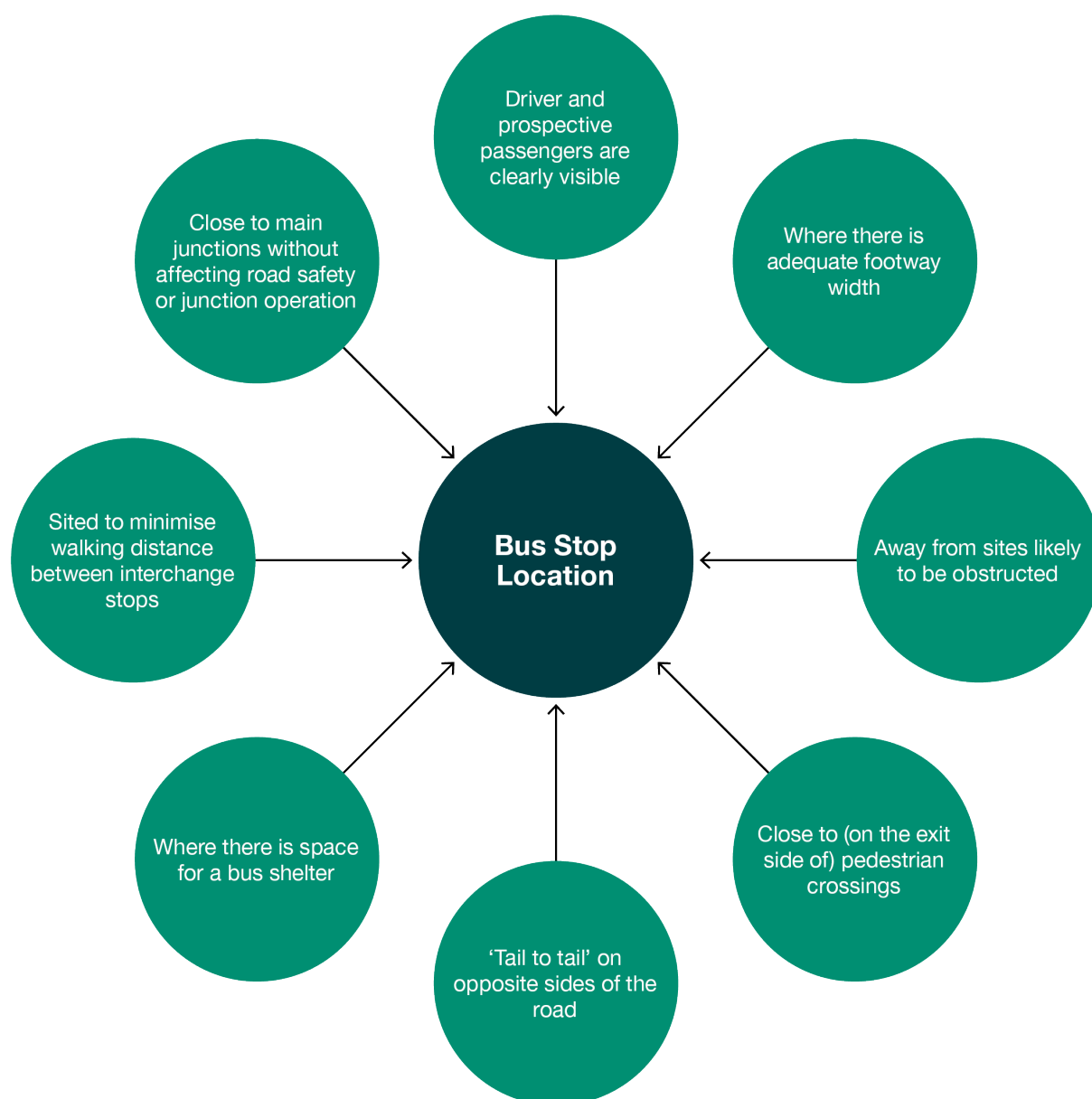
(Figure 5: considerations for bus stop locations (TfL accessible bus stop design guidance 2006))
